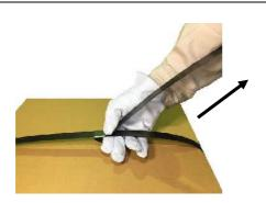
③ Tighten the strap passed through the seal in the arrow direction to remove excess looseness.
