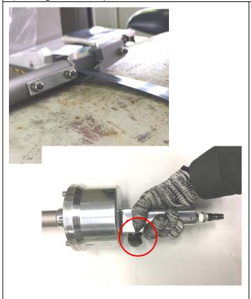
4 While holding the cutter in a set state, push the valve button with your index finger to cut the strap.
