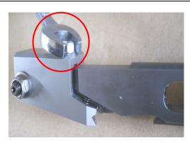
② Loosen the nut, and turn the gripper angle adjustment bolt to make an adjustment.
