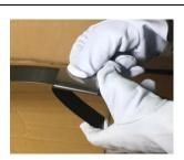
② Pass the end of the strap through in the seal. Then, fold the end of the strap under the seal (folding length is approximately 50mm)
